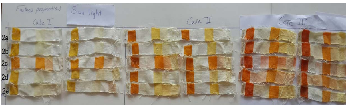
Plate (3): Light fastness outdoor exposure to sun light
