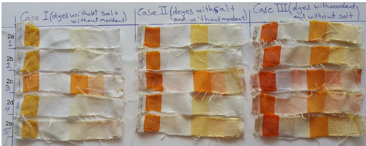
Plate (1): Dyeing a multi-fiber strip in cases I, II, and III
