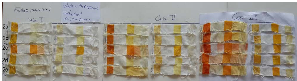
Plate (5): Wash and rubbing fastness of dyes in a cationic surfactant solution
